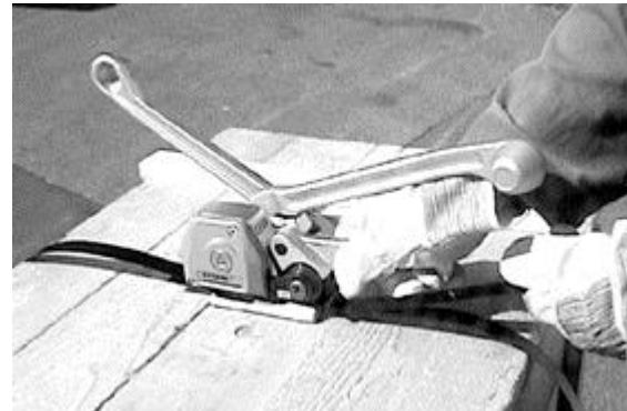
The right hand grasps the tension lever **508** and moves it back and forth to obtain the desired strap tension. At the same time the left hand holds the cutting lever **511**.
