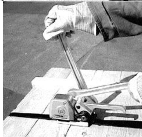
After having reached the desired strap tension bring tension lever **508** back into its initial position. The right hand remains there and provides support for the joining process. The TITAN "No-seal" joint is formed by pushing the cutting lever **511** forwards rapidly with the left hand until it strikes against the case; the steel strap is simultaneously cut off directly behind the joint.
