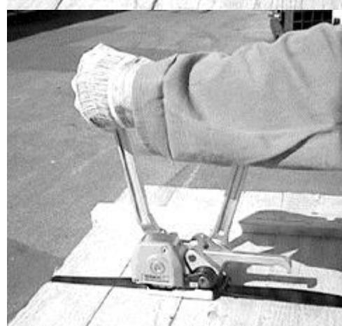
Bring tension lever **511** back into its initial position. Grasp and press together rocker **509** with cutting lever **511**. Withdraw the tool from the package by a rotary movement to the right side.
