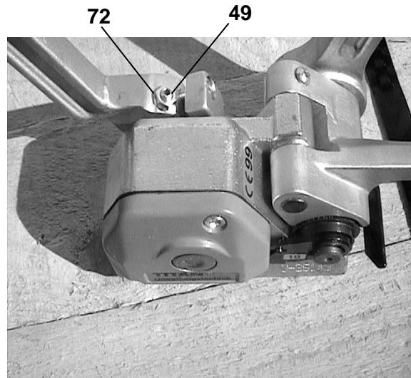
Fasten hexagon nut **72** after adjustment has been completed.
