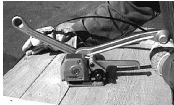
2. Pull through the strap end until it is in the centre of the package beneath the upper run of strap and juts out approx. 15 cm.
