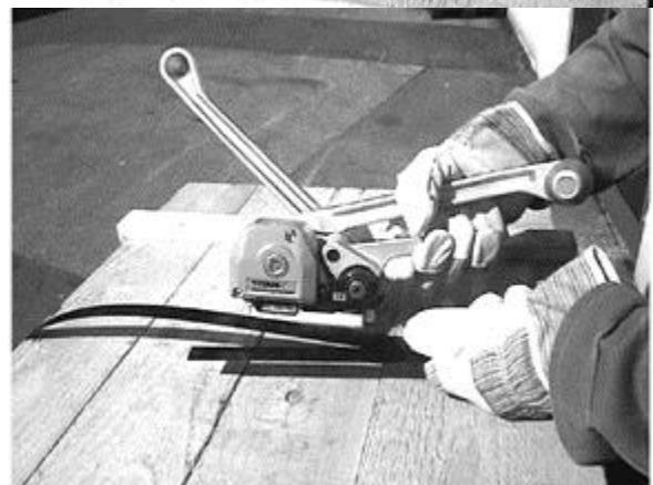
3. With the left hand hold the upper and lower run of the strap together. Both straps must be placed exactly on top of one another. Grip and press rocker **509** together with the cutting lever **35** with the right hand. Insert the steel strap laterally until it strikes against the case wall, ensuring that the lower run of strap projects slightly out of the tool at the front. The right hand now releases the levers which have been pressed together.
