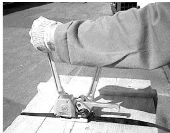
7. Bring tension lever **508** back into its initial position. Grasp and press together rocker **509** with cutting lever **35**. Withdraw the tool from the package by a rotary movement to the right side.
